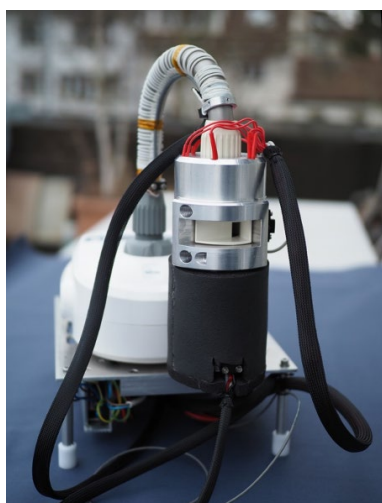
Figure 2: Aerosol sampler modified for operating at high altitude
